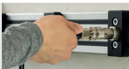
One-hand operation: Connection through simple pushing the plug into the coupling
