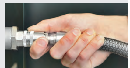
To disconnect, slide the sleeve back (with automatic locking mechanism)
