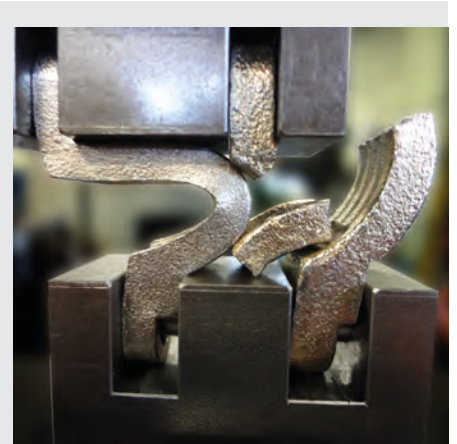
Distance of 23 mm (no cracks in the LUDECKE hose clamp, completely destroyed counterfeit)
