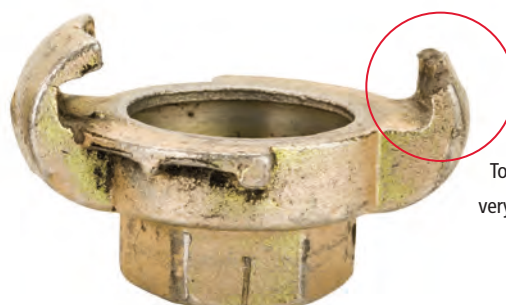
Counterfeit from the Far East (no manufacturer's branding, inferior material)
