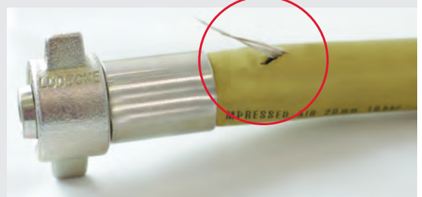
Busted hose - LUDECKE -fitting incl. assembly hold
