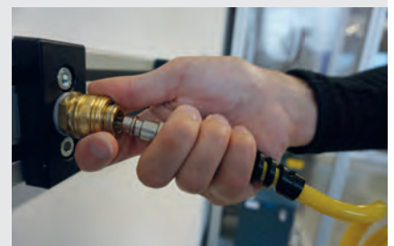
To disconnect, slide the sleeve back, whilst the locking mechanism (ball or pin locking) opens automatically and hold the plug
