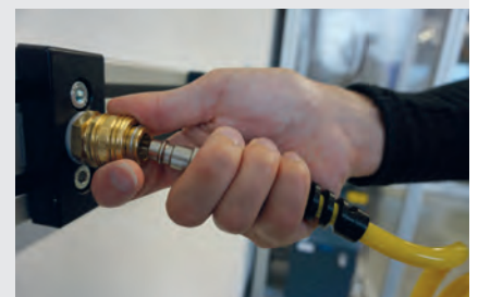
To disconnect pull back the sleeve of the coupling (ball or pin locking opens automatically and releases the plug)
