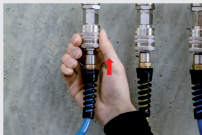
Disconnection - first step: Automatic venting
