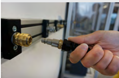
One-hand operation: connection through simple pushing the plug into the coupling.
